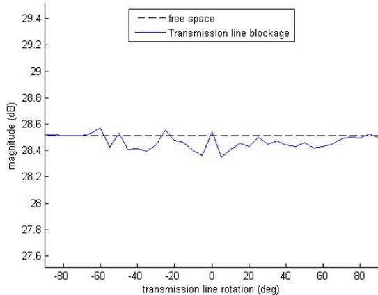
**Figure 8 - Dipole looking through transmission Line structure**
