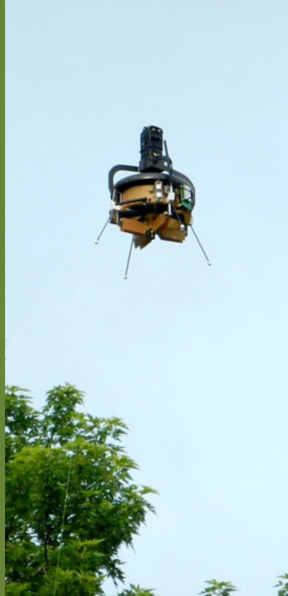
HARC-Tethered Drone uses a ducted-fan vehicle to achieve 30% more lift and safer handling ▶
