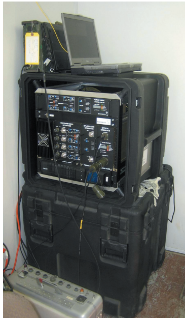
A radio antenna aboard a HARC aerostat is connected to a radio interface unit on the ground. Forax technology allows the radio's analog signal to be carried via fiber without digitization.
