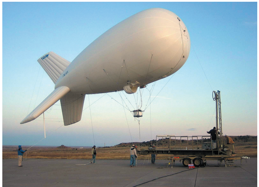
Technicians launch an aerostat containing a High Antennas for Radio Communications, or HARC, payload. An optical fiber tether carries an analog ground radio signal to its corresponding antenna aboard the aerostat, providing greatly increased transmission range.
