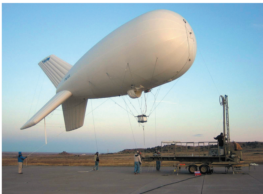
Technicians launch an aerostat containing a High Antennas for Radio Communications, or HARC, payload. An optical fiber tether carries an analog ground radio signal to its corresponding antenna aboard the aerostat, providing greatly increased transmission range.
