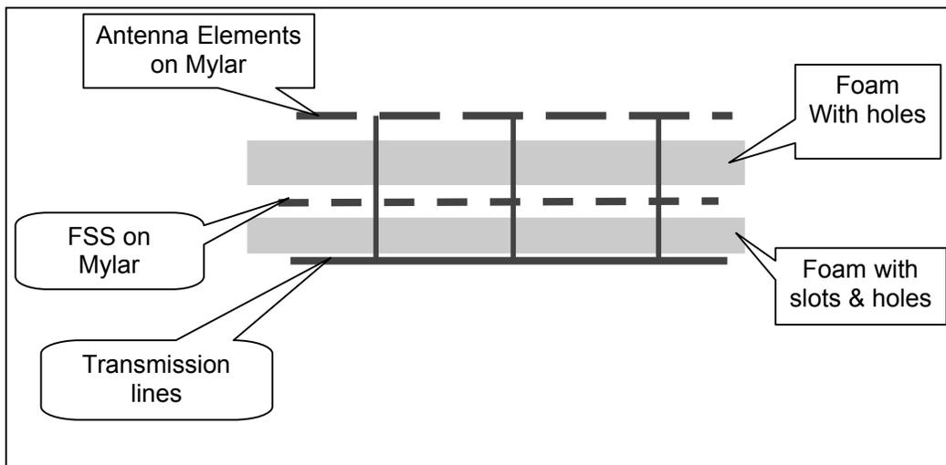
**Fig. 2. Side diagram of an individual array**
