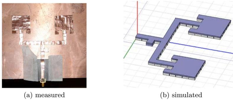
Figure 2: 2 element array on finite substrate
