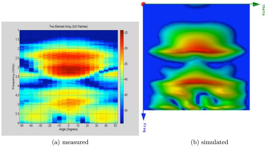
Figure 4: Radiation intensity vs. gain and elevation
