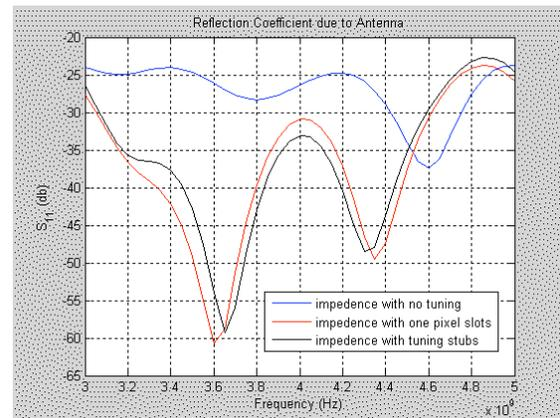
Figure 4. Pixel patch antenna  $S_{11}$  values.
