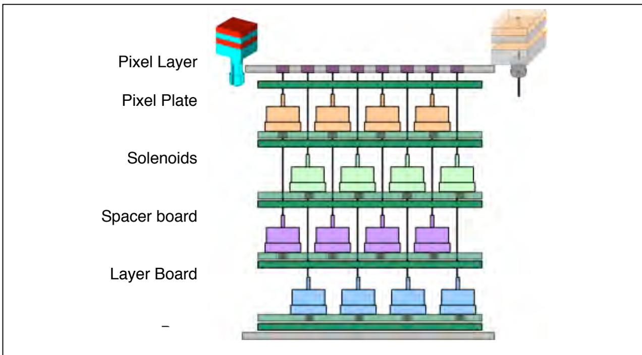
Figure 6. Solenoid configuration on 4-layer PC boards.
