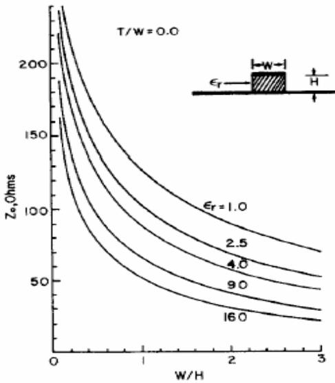
Figure 2. Finite dielectric Microstrip lines (from [4])
