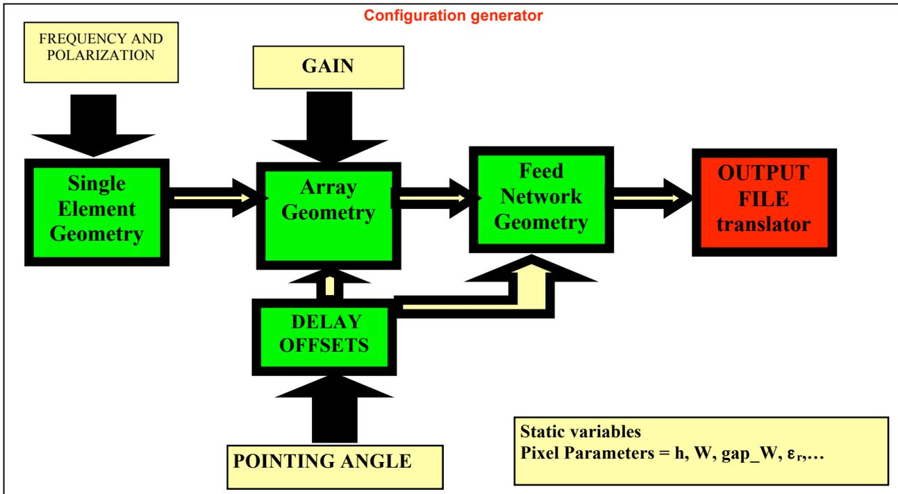
Figure 7. Logic flow diagram for automatic antenna array generation using pixels.
