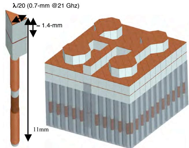
Figure 1. Ceramic pixel microstrip concept
