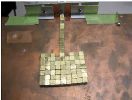
Figure 3. Patch antenna from 1/4 inch square pixels
